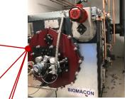
Syngas-heated reactor – S representative of Pyreg or BioMaCon units
